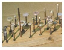
This is an assortment of tool tips I made using the government issued copper penny for some. All the mandrels are made of 1/8" welding rod. The tips are soldered onto the mandrels using silver solder.
