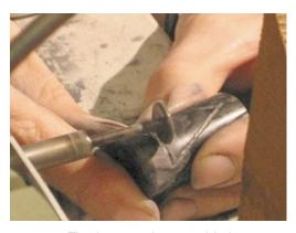
The images above and below were made using the copper wheel to grind and polish the grooves. The grit used was traditional emery in grades 200 and micro grit and finished with pumice.
