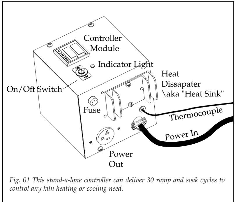
Fig. 01 This stand-a-lone controller can deliver 30 ramp and soak cycles to control any kiln heating or cooling need.
