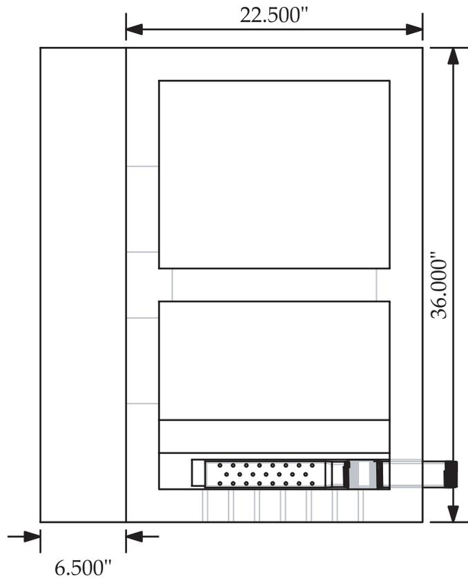
This is the body of a garage. The exterior of the shape measures 36" x 22.5" in the top view with a 6.5" shelf. the walls are 2.5" thick made of IFB. These dimensions were taken from a functional garage built by Charles Correll. His did not have a baffle structure in the center of the garage. He felt the design, as he built it, worked fine but the heat loss was great which is something to consider with the price of fuel today.
