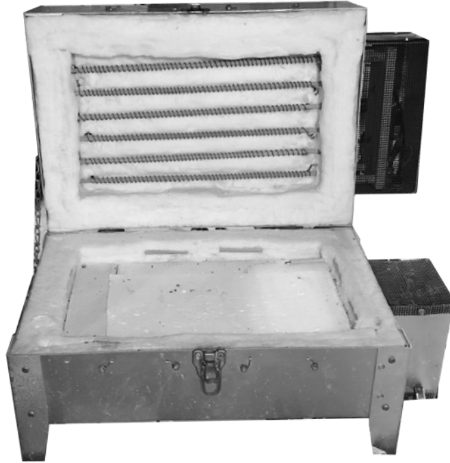
Fig 7 These are the element segments as photographed on November 2, 2025 showing the 100% success of this approach to this ceiling install in a fiber blanket kiln. I have not made a single adjustment in these elements in their 11-1/2 years of service.
